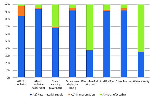
Figure 2. Potential environmental impact contribution per metric ton of steel WF beam
