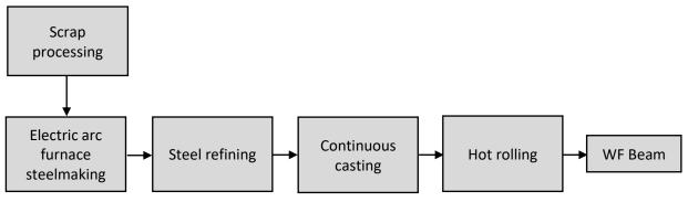
Figure 1. Flow diagram of steel WF beam manufacturing process
