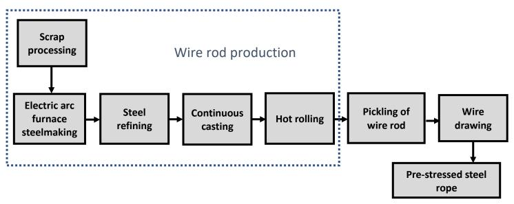
*Figure 1. Flow diagram of the manufacturing process of pre-stressed steel rope.*
